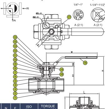
SIZE W H1 H2 F Н М N DN 5211 in-lbs NM 1/4' 8 11.0 75.7 68 131 9 36.8 8.2 6 6 76.5 F03/F04 292 33 131 3/8" 10 11.0 75.7 68 9 36.8 8.2 6 6 76.5 F03/F04 292 33 1/2' 131 440 50 15 86.6 74 F03/F04 16.0 9 44 1 90 6 6 894 3/4" 94 184 800 90 20.0 103.0 11 55.1 11.5 6 101.6 F04/F05 1" 25 100 184 60.7 11.5 115.4 F04/F05 1504 170 25.0 118.2 1-1/4" 1950 220 32.0 125.8 75.2 15.1 125.2 F05/F07 38.0 149.0 123 227 84.4 F05/F07 3360 380 1-1/2" 14 15.1 148.6
